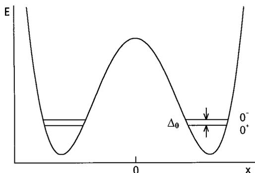
FIG. 2. Schematic diagram of the double minimum potential for the proton tunneling motion of tropolone (one-dimensional model). The lower and upper components of the tunneling doublet in the ground vibrational state are denoted by  $0^+$  and  $0^-$ , respectively, and their energy separation by  $\Delta_0$ .
