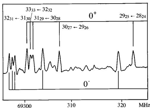
FIG. 3. Rotational transitions observed at around 69.3 GHz both for the  $0^+$  and  $0^-$  states. Asymmetry doubling is not resolved for these lines. The  $J_{K_c} = 33_{33} - 32_{32}$  line, e.g., consists of the two unresolved asymmetry doublet components,  $33_{0,33} - 32_{0,32}$  and  $33_{1,33} - 32_{1,32}$ .
