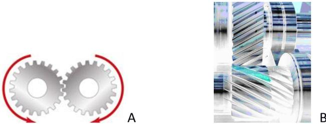
Instead of the gears as in the image A, we imagine two helical gears with opposite teeth as in the image B. If both have their own drives, they complement each other, i.e. these two forces add up no matter whether they are of equal or of different intensity.
