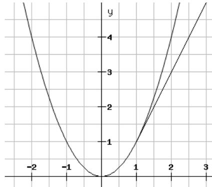
As we have said, we assume  $\Delta x$  to be very small, practically zero, so only  $2x$  remains for the steepness. We see that the steepness is a continuous function as well as the basic function, which one could have expected. This means that for any given point  $x$  we can now not only specify the value of the function, but also of the steepness at that point.
